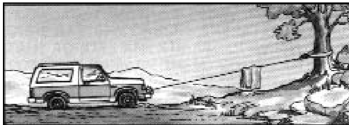
For basic self recovery, anchor to a tree or heavy rock. When anchoring to a tree, always use a tree trunk protector.
