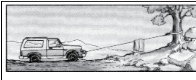
For basic self recovery, anchor to a tree or heavy rock. When anchoring to a tree, always use a tree trunk protector.
