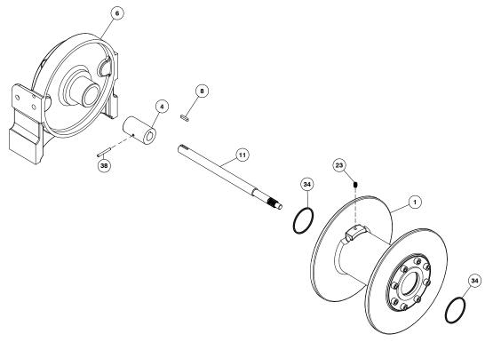
9. If splines inside drum driver #102 are damaged, drum driver must be replaced. Remove drum driver by unscrewing (8) capscrews #105. If bushings show signs of wear, replace by pressing old bushings from drum #101 and removing o-rings from grooves in drum and drum driver. Place well oiled o-rings #106 into driver and drum. Place well oiled o-ring #107 on outside of driver. Press bushings #104 into drum driver until flange is flush and #103 is flush against drum.
