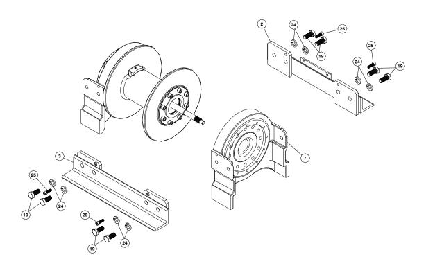
8. Pull drum assembly #1 from end bearing #6. Remove quad-rings #34 from grooves in drum bushings. Remove input shaft #11 from end bearing. Examine splined ends of input shaft for signs of wear, replace if damaged. Examine drum assembly #1 for signs of wear.
