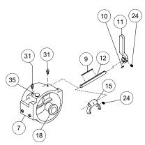
11. Check cover bushing (item #18) for signs of wear. If necessary remove old bushing and press bushing into place.
