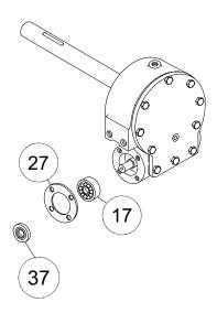
15. Place gasket (item #27) onto adapter (item #1). Slide seal (item #37) onto worm. Slide tapered end of coupling (item #25) over end of worm shaft. Attach adapter and coupling to gear housing using four screws (item #21). Tighten screws to 12 ft-lbs. (16.3 Nm) each.
