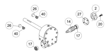
Remove gear housing cover (item #4) from gear housing (item #8) by unscrewing capscrews (item #20).
