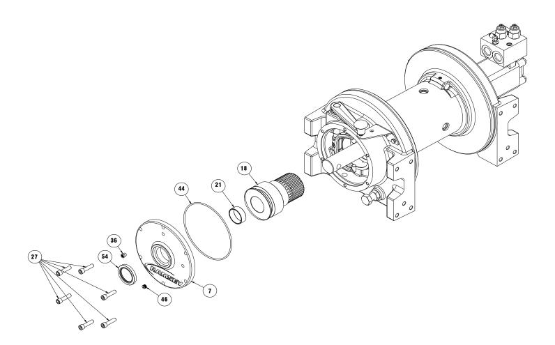
4. Slide clutch end bearing #2 from drum. Drum freespool drag puck #12, drum freespool spring #58, and brake disc spacer #62 will fall out when end bearing is removed from drum. Retain these items for re-assembly.
