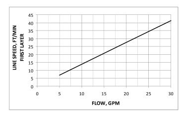
BASED ON 14.9 CU IN/REV MOTOR
