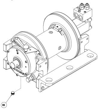
2. Freespool drum to locate drain hole in bottom. Remove plugs #47 from barrel of drum. Drain oil from drum barrel. **When refilling oil in drum, use 16 ounces of SAE 75W-90**. Remove mounting angle #5 by loosening (3) capscrews #25 each side.
