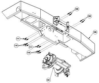
5. Remove vertical roller pin #120 from right hand side of roller guide #102 by removing spring pin #119. Spring pins should be removed by driving inward through the roller. Vertical roller pin has (2) lube fittings #118 located one at either end of the roller. Once the vertical roller pin is removed from right hand side of roller guide, vertical roller #117 can be removed. Remove vertical roller from left hand side of roller guide in the same way.
