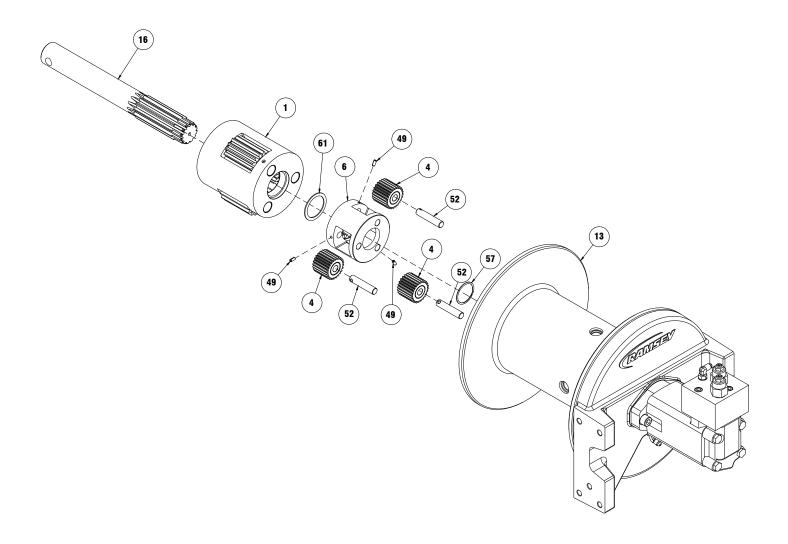
7. Remove drum #13 from motor end bearing #3. Remove drum seal #55. Check for signs of wear and replace if necessary.
