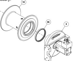
8. Remove input shaft #14 from motor end bearing #3.
