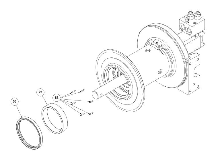
6. Remove output shaft #16, output carrier assembly #1, and input carrier assembly #6 from drum #13. Disassemble in the following order:
