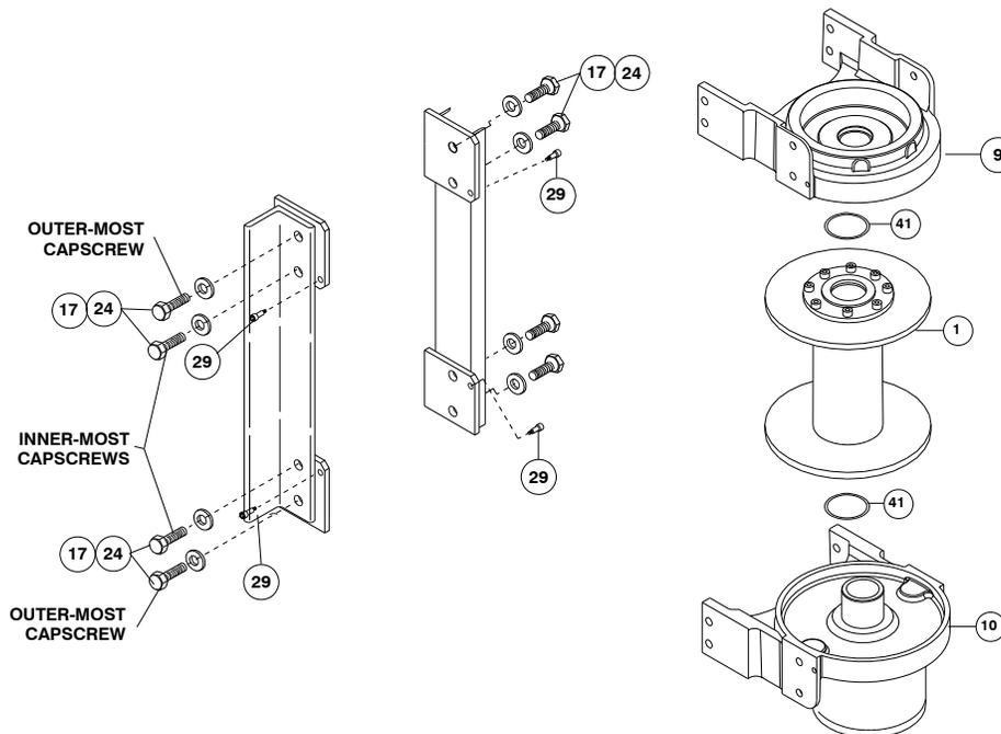
9. Place end (with longest splines) of output coupling #8 through end bearing bushing #13 and mesh coupling spline with spline inside of drum. Slide clutch spacer #30 over end and against shoulder of shifter shaft #12. Place shifter shaft through washer #27 and into shaft coupling #6, meshing splines of shifter shaft with splines in shaft coupling.
