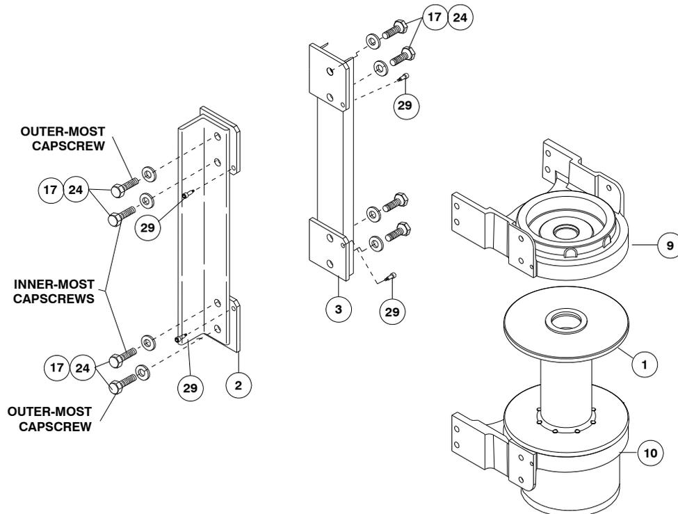
5. Pull drum assembly #1 upward from end bearing #10. Remove quad-rings #41 from grooves in drum bushings. Remove input shaft #11, clutch springs #44 & #45 and washers #27 & #28 from end bearing. Examine splined ends of input shaft for signs of wear, replace if damaged.
