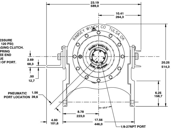
WITH PLUG AND CARTRIDGE IN POSITION SHOWN CABLE DRUM ROTATES CLOCKWISE, AS VIEWED FROM MOTOR END OF WINCH, TO REEL CABLE IN. LOCATION OF PLUG AND CARTRIDGE MUST BE REVERSED FOR OPPOSITE ROTATION
