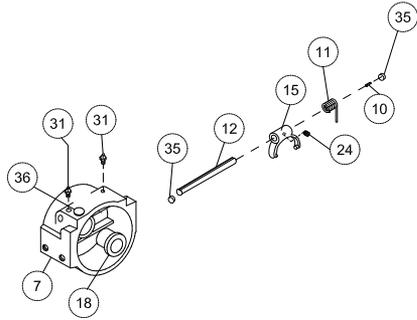
11. Check cover bushing (item #18) for signs of wear. If necessary remove old bushing and press bushing into place.
