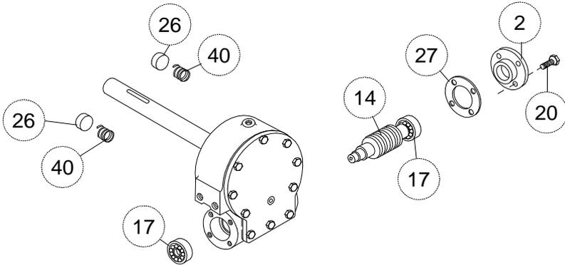
6. Remove gear housing cover (item #4) from gear housing (item #8) by unscrewing capscrews (item #20). Thread two of the capscrews into the two tapped holes of cover and tighten. This will pull the cover loose from the gear housing.
