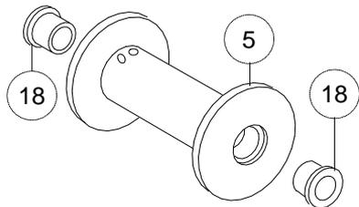
10. Check clutch housing bushing (item #18) for wear. If necessary, remove old bushing and press new bushing into place. Check yoke (item #15) for damage. Yoke should be firmly attached with setscrew (item #24). Apply grease to lube fittings (item #31) to lubricate clutch shifter shaft (item #12).
