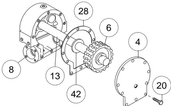
13. Press bearing (item #17) onto worm (item #14) Note: Be sure that thick shoulder of bearing's outer race (side with manufacturer's name and part number) is out, away from worm threads. Press bearing and worm into gear housing. Slip gasket (item #27) onto bearing cap (item #2). Use four cap-screws (item #20) to secure cap to gear housing. **Tighten capscrews to 8 ft-lbs. (10.8 Nm) each.**
