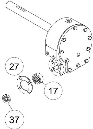
15. Place gasket (item #27) onto adapter (item #1). Slide seal (item #37) onto worm. Slide tapered end of coupling (item #25) over end of worm shaft. Attach adapter and coupling to gear housing using four screws (item #21). **Tighten screws to 12 ft-lbs. (16.3 Nm) each.**
