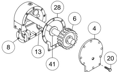
7. Check for signs of wear on gear teeth. If replacement of gear is necessary, replace as follows:
