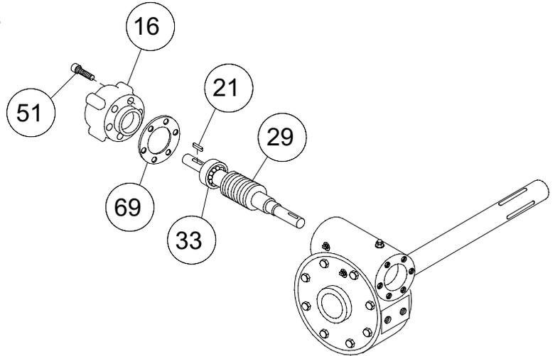
Slip gasket (item #69) onto brake housing (item #16). Use (6) capscrews (item #51) to secure brake housing to gear housing. Tighten capscrews to 45 ft-lbs. (61 Nm) each.
