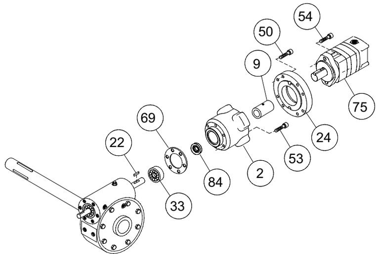
Insert key (item #22) into keyway of worm shaft. Slide coupling (item #9) over end of worm shaft. Attach adapter plate (item #24) to adapter using (8) capscrews (item #50). Tighten capscrews to 21 ft-lbs (28 Nm) each.
