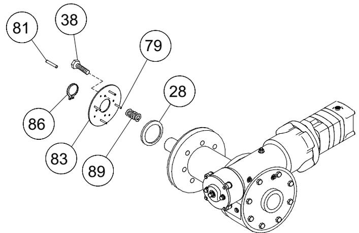
**NOTE:** If roll pins (items #79 and #81) are damaged, remove and install new pins as follows:
