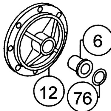
13. Apply grease to end of shaft, opposite gear. Apply grease to bushing in gear housing (item #18). Place greased end of shaft through bushing in gear housing. Place gasket (item #71) onto gear housing cover (item #12). Apply grease to gear end of shaft and cover bushing. Place cover onto shaft and secure to housing with (8) capscrews (item #42). Tighten capscrews to 39 ft-lbs. (52 Nm) each.
