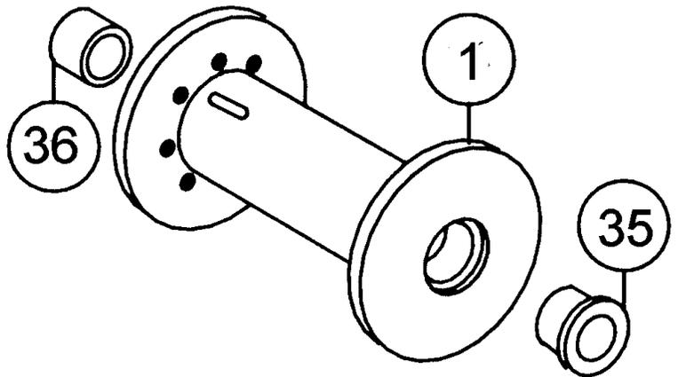
11. Check end bearing bushing (item #36) for signs of wear. If necessary, remove old bushing and press new bushing into place.
