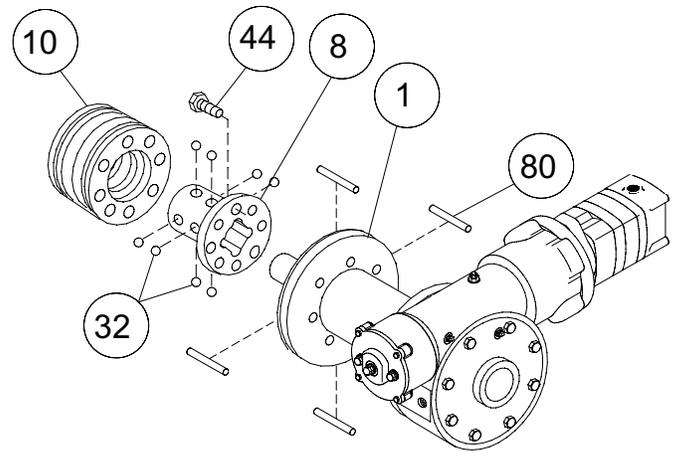
Rotate the drum to align the clutch slots with the shaft keyways. Lightly grease (4) dowel pins (item #80) and (8) balls (item #32) with molybdenum disulfide or graphite bearing grease. Insert the dowel pins and balls. In the engaged position the balls are nearly flush with the clutch.
