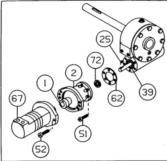
16. Press bearing (item #39) onto worm and into housing. **NOTE:** Be sure that thick shoulder of bearings outer race (side with manufacturer's name and part number) is out, away from worm threads. Attach adapter (item #2) to gear housing using six capscrews (item #51). Tighten capscrews to 12 ft. lbs. (16.1 Nm.) each. Insert key (item #25) into keyway of worm shaft. Slide tapered end of coupling (item #1) over end of worm shaft.
