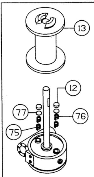
17. Place winch with gear housing cover down on work bench. Drum shaft should be in vertical position. Set springs (items #75 & #76) into pockets of gear housing with drag brakes (item #12) on top of disc (item #77) and springs. Slide drum assembly (item #13) onto drum shaft with drum jaws upward.
