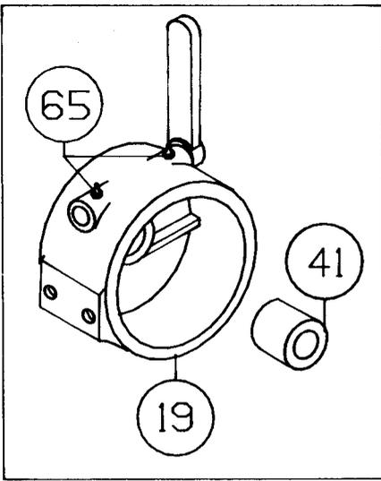
11. Check clutch housing bushing (item #41) for wear. If necessary, remove old bushing and press new bushing into place. Apply grease to lube fittings (item #65) to lubricate clutch shifter shaft.
