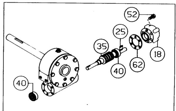
15. Press bearing (item #40) onto worm and into gear housing. **NOTE:** Be sure that thick shoulder of bearings outer race (side with manufacturer's name and part number) is out, away from worm threads. Attach bearing cap (item #8), to gear housing. Use six (item #44) capscrews to secure. Tighten capscrews to 18 ft. lbs. (24.4 Nm.) each. Tap key (item #25) into keyway.
