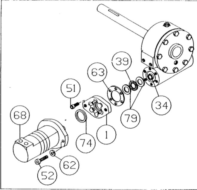
5. Refer to page 3, SERVICING OIL COOLED SAFETY BRAKE. Remove brake housing (item #18) from gear housing by unscrewing six (item #52) capscrews. Remove worm (item #35) and bearings (item #40) from gear housing. Use a soft hammer to gently tap input end of worm and drive worm and bearing from gear housing. Once worm has been removed from housing, bearing can be pressed from end of worm.
