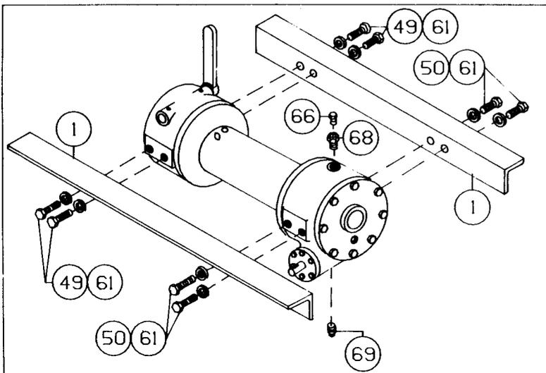
19. Attach two mounting angles (item #1) using four (item #49) capscrews with lockwashers at clutch housing end and four (item #50) capscrews with lockwashers at gear housing end. Torque capscrews to 28 ft. lbs. (37.9 Nm.) each. Insert plug (item #69) into bottom of gear housing. Permatex may be applied to threads to help prevent leakage.
