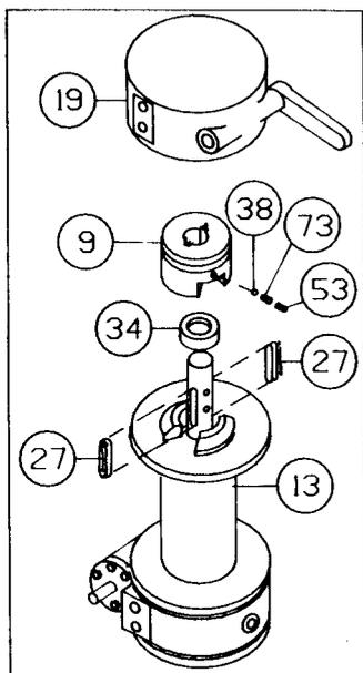
2. Slide clutch housing (item #19) from end of drum shaft. Remove setscrew, spring and poppet ball (items #53, #73 and #38) from jaw clutch (item #9). Slide jaw clutch from end of drum shaft.
