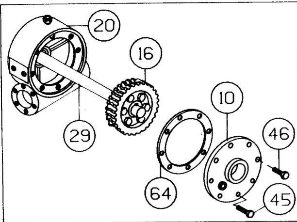
13. Apply grease to end of shaft, opposite gear. Apply grease to bushing in gear housing (item #20). Place greased end of shaft through bushing in gear housing (item #20). Place gasket (item #64) onto gear housing cover (item #10). Apply grease to gear end of shaft and cover bushing. Place cover onto shaft and secure to housing with seven (item #46) and one (item #45) capscrews. Tighten capscrews to 12 ft. lbs. (16.1 Nm.) each.
