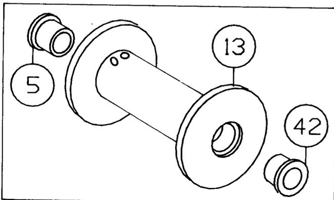
10. Check drum bushings (items #5 & #42) for signs of wear. Replace if necessary by pressing old bushings from drum. Press new ones into place.
