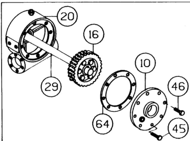
6. Remove gear housing cover (item #10) from gear housing (item #20) by unscrewing capscrews (items #46 & #45). Thread two of the capscrews into the two tapped holes of cover and tighten. This will pull the cover loose from gear housing.
