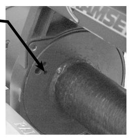
4. Feed synthetic rope through aluminum hawse fairlead and under drum. See figure page 4.
