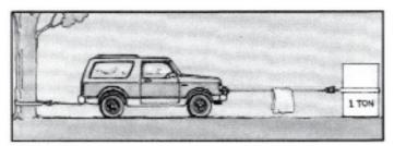
For a direct pull of 2000 lbs., hitch truck to a tree or solid anchor, and take out of gear. To double the pull, use 2-part line and tie off to chassis.
