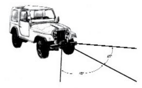
Winches equipped with fairleads can pull from several directions. Pull from an angle only to straighten up the vehicle-otherwise you can damage structural members or other parts of your vehicle and cause excess rope buildup on one end of the winch drum.
