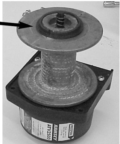
3. Remove the bolts that hold the end plate to the motor end housing. Lift off the end plate and take the nuts and washers out of the mounting feet. Set aside the gear assemblies and bushing. The input sun and planetary gear carrier may come out together.
