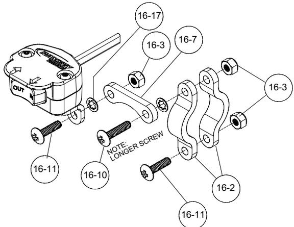
4. Install the Mounting Arm (item #16-7) to the Handle Bar Clamps using a 7/8" long #10 screw (item #16-10), shake-proof washer (item #16-17), and locknut (item #16-3). Install the shake-proof washer between the handle bar clamps and the mounting arm. See figures at left. Do not tighten.
