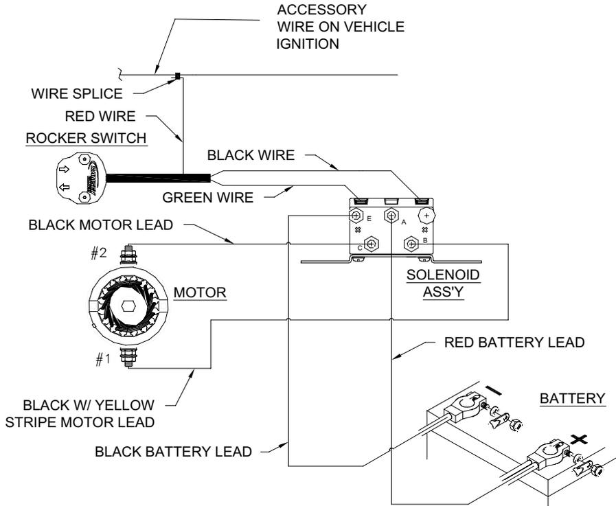
**For certain mounting applications,** where the solenoid needs to be mounted at the rear of the vehicle, switch the battery and motor leads. In this case, connect the black w/yellow stripe lead to the positive (+) terminal of the battery, and the longer black lead to the negative (-) terminal. Connect the red lead and the shorter black lead to the motor terminals.
