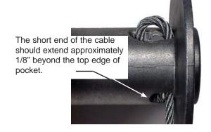
Slide the cable through narrow end of the pocket against drum flange and wrap the cable around the anchor puck. Pull the cable and anchor back into the wide end of the pocket leaving approximately 1/8" beyond edge of pocket as shown. Use a hammer and drift punch to drive the back side of the wire rope, firmly seating the wire rope and anchor into the pocket.
