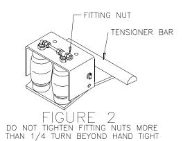
drum, watch the tensioner. Tensioner must be free to move without obstruction to function properly. If tensioner touches any surrounding structure, correct the problem.
